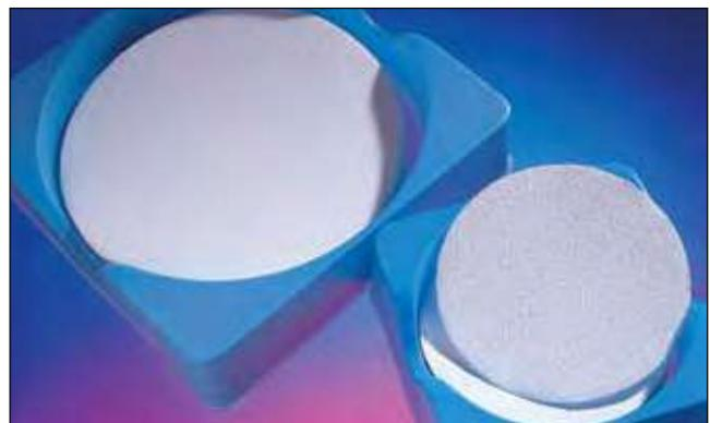
These acid treated low metal filters are available in 47, 90, 110, 125, 142, and 150 mm diameters. The 90 mm filter is required for volatile samples and use with a Zero Headspace Extractor.
