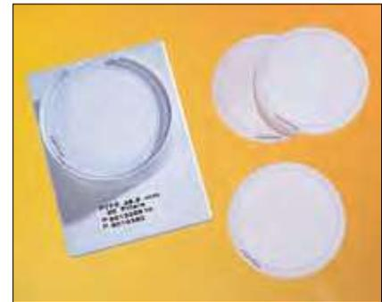
These include trace metal analysis by XRF and visual inspection for defects such as pinholes, support ring separation, chaff or flashing, loose material, discoloration, filter nonuniformity or any other obvious filter defect.
