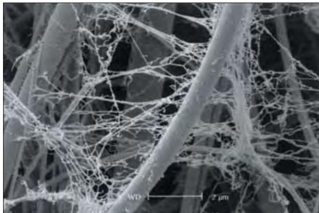
Electron micrograph showing DNA entrapped within the FTA matrix (magnification  $\times 10,000$ )
