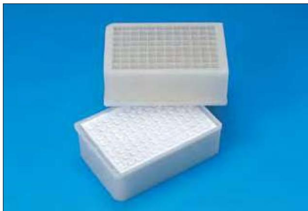
Glass-filled polypropylene 96 well UNIFILTER
