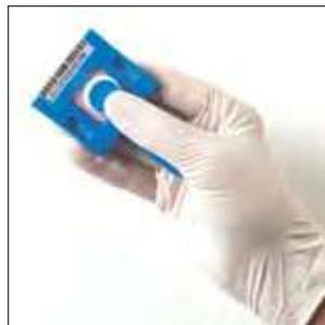
Close the device to transfer cells to the Indicating FTA Card; ensure the foam applicator is snapped into place.
