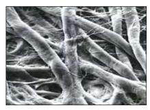
Whatman cellulose filter papers exhibit particle retention levels down to  $2.5 \mu m$ .
