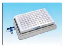
UniVac 1 vacuum to waste manifold
