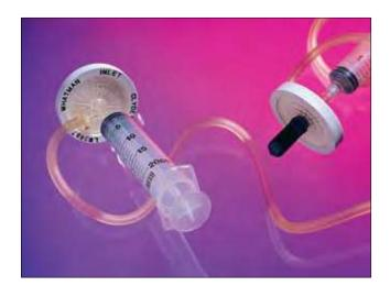
Clyde can be used with tissue culture media and aqueous solutions compatible with the cellulose membrane. As Clyde needs no vacuum pump or other power supply, field work applications are also possible.
