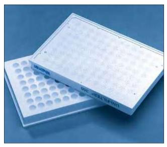
96 well UNIFILTER microplate: mesh bottom
