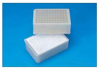
Glass-filled polypropylene 96 well UNIFILTER
