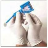
Peel off the protective film exposing the Indicating FTA Card.
